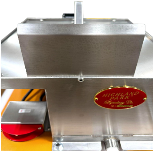
Proper Splash Guard Installation
