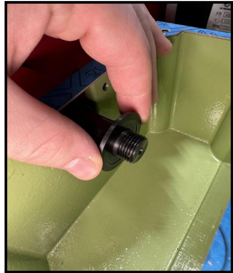
Place 1st flange flat side against arbor shaft, recessed side against blade.
