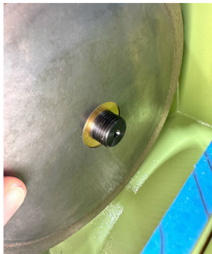
Be sure the bushing is centered both inside the blade and on the arbor.
