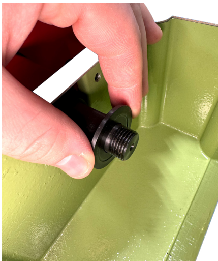
Place 1st flange flat side against arbor shaft, recessed side against blade.
