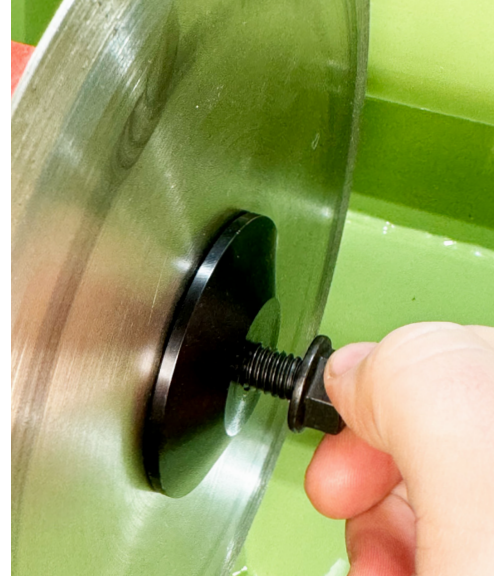
Place second flange with the recess against the saw blade and secure with the arbor nut.
