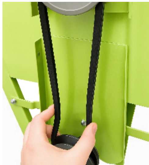
Testing Belt Tension
