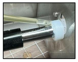
and begins to slip on the drive rollers (which could happen after extended use), the exterior can be roughed up a little by hand using some 400 grit sandpaper, which will allow it to grip the rollers better.
